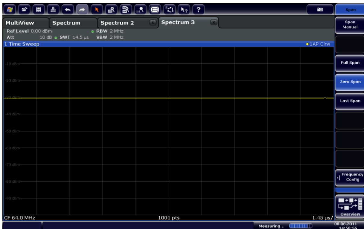
Fig. 4-7: Time domain display of the calibration signal
